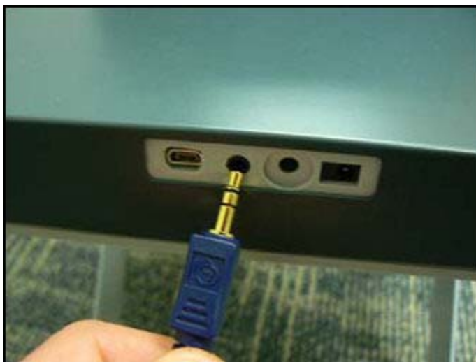
Figure 137. Plugging the Remote Trigger Cable Into the Portable Test Stand
