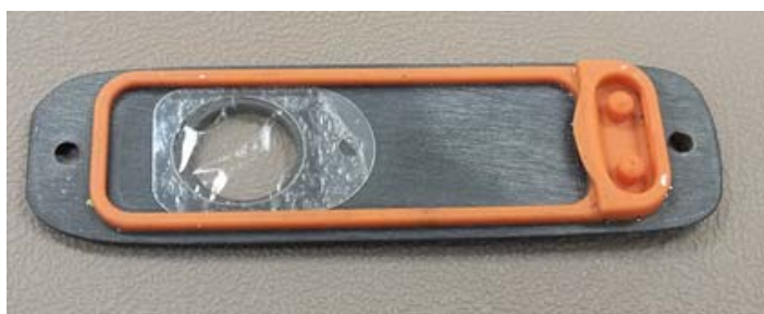
Figure 127. Measurement Window Replaced
