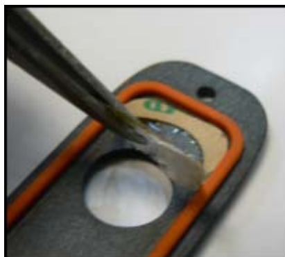
Figure 124. Removing the Old Window
