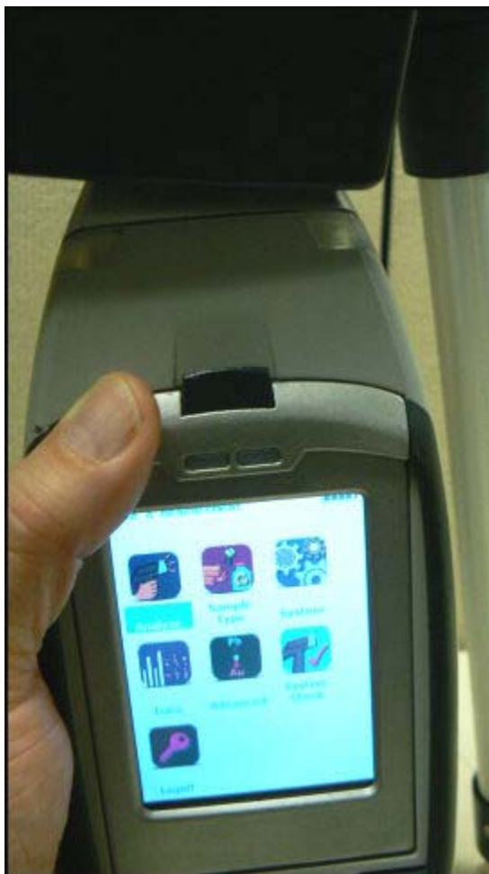
Figure 146. Inserting Analyzer into Portable Test Stand
