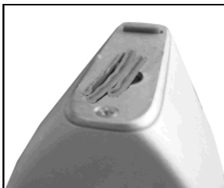
Figure 46. PVC Wire Insulation With Conductor Removed
