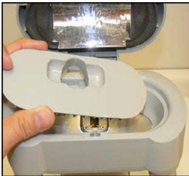
Figure 150. Inserting the Sample Cup Holder
