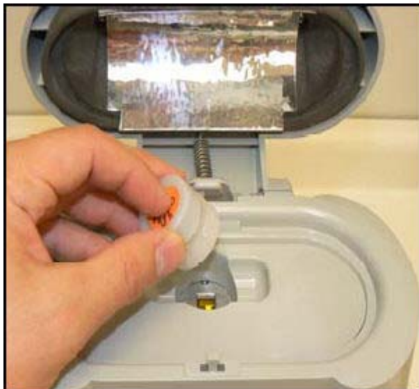
Figure 151. Inserting Sample Cup
