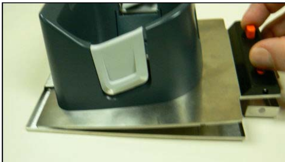
Figure 160. Inserting the Top Plate into the Test Guard
