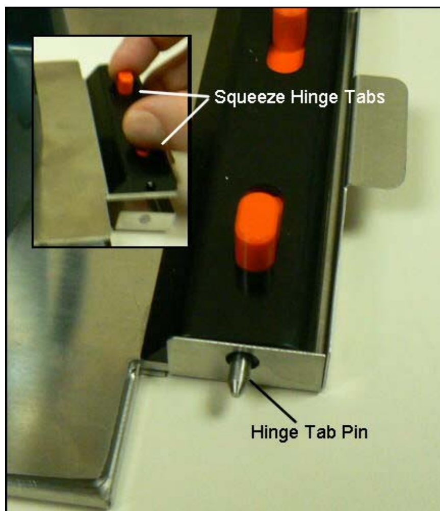
Figure 162. The Hinge Tab Pins
