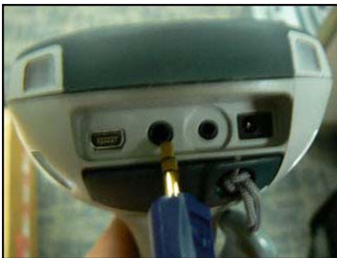
Figure 138. Plugging the Remote Trigger Cable Into the Analyzer
