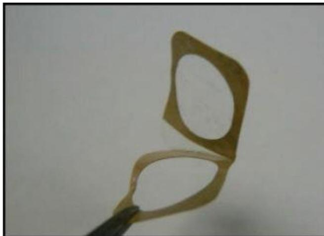
**Figure 73.** Removing the Backing from Prolene Window
