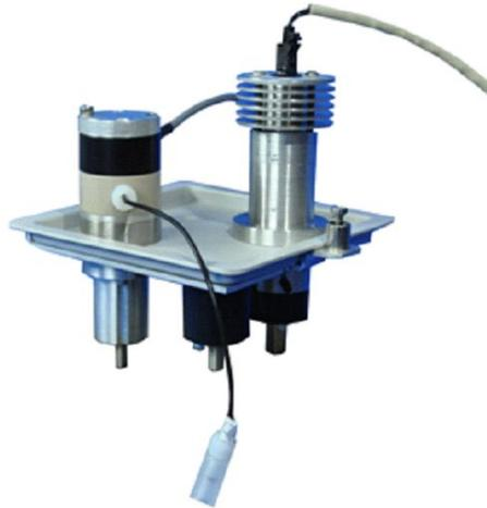
**Figure 3.16.** Photometric Detector Assembly
